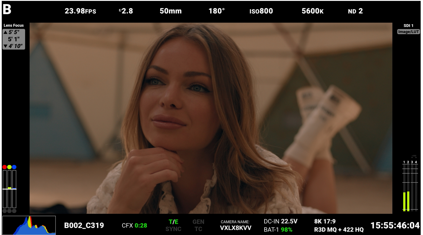
Figure: SDI monitor with SDI Technical Overlay Mode enabled
