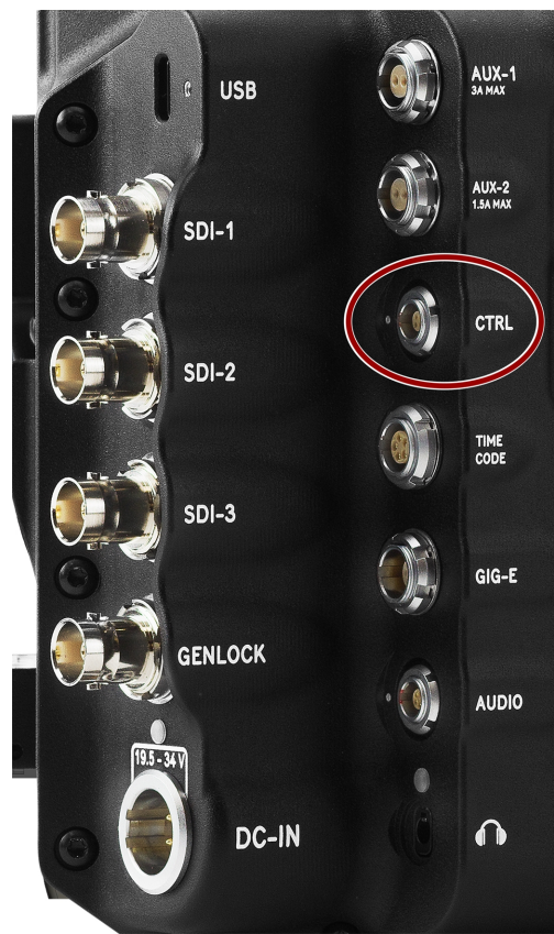
Figure: Front face of female 4-Pin 00B CTRL connector (looking at the back of the camera).
